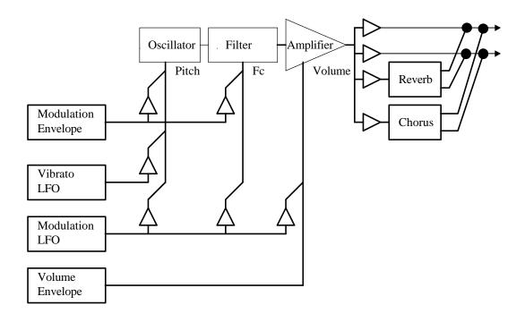
**Figure 2: Generator Based Modulation Structure**
