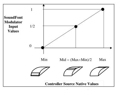
**Figure 5: Positive Unipolar Linear Plot**
