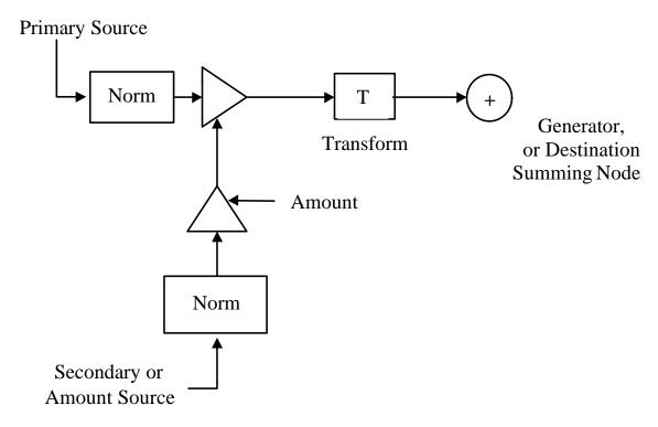
Figure 3: SoundFont Modulator Building Block
