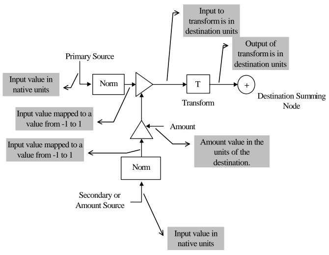
**Figure 4: Detailed SoundFont Modulator Building Block**
