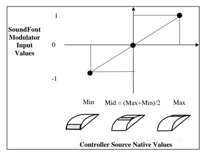
Figure 6: Positive Bipolar Linear Plot
