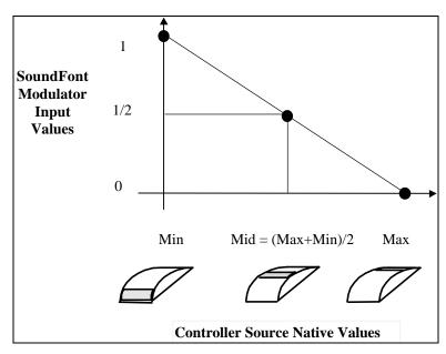
**Figure 7: Negative Unipolar Plot**
