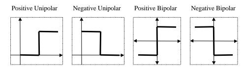
**Switch Controller Curves** for given Directions and Polairities
