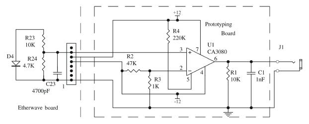
Figure 7 - Output Amplifier for Tuner
