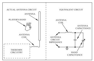
Figure 1 - Equivalent Circuit of Hand Capacitance
