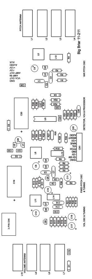
Figure 4 - Component Layout of Etherwave Circuit Board
