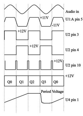
Figure 11 - Pitch CV Circuit Waveforms
