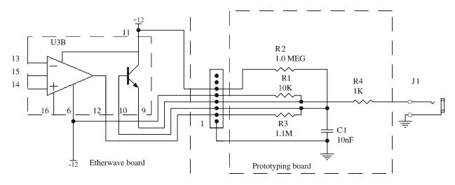
Figure 9a - Etherwave Volume CV Circuit
