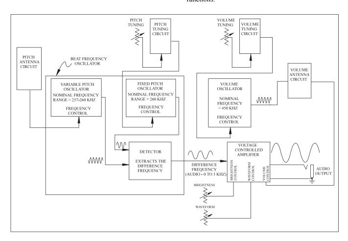
Figure 2 - Etherwave Block Diagram
